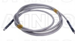
1.85M-1.85F-B010S-3000 Flexible Cable Assembly 3000mm DC-67GHz 1.85mm Male to 1.85mm Female
